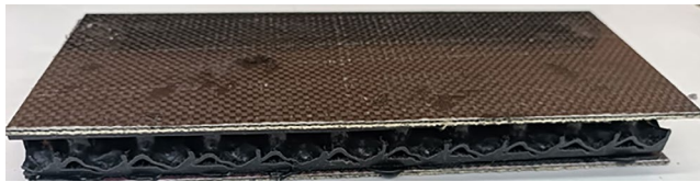
FIGURE 3 | Isometric view of the produced sandwich composite structures.
